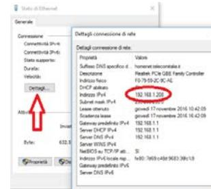
connection details with the IPv4 address. In our example our IPv4 is 192.168.1.208; in order to have your MCP communicating with your PC is necessary to assign an IP number to your MCP. As default the MCP has the IP address 192.168.1.40. So is not necessary to assign any new IP number. If the two IP addresses would be identical it will be necessary to modify the MCP IP address. How to do it will be explained in the programming section.
