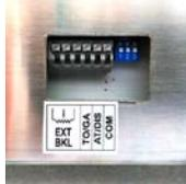
**EXTERNAL TO/GA:** External TO/GA can accept input from a pushbutton. The pushbutton contact must be open in normal condition and close only when pressed, do not connect steady position switches to this input. The TO/GA function engaging depends by the aircraft
