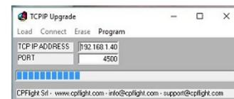
At the end it will appear a window that indicates the end of the programming. Close the upgrade program and disconnect the power supply from the MCP. Connect another time the power supply to verify that in the IAS display window of your MCP will appear the new release number.
